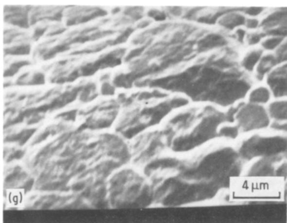
*Figure 1* SEM micrographs of AP pellets compacted at  $1500 \text{ kg cm}^{-2}$  at various dwell times (a, b) microstructures of 0 min compact at  $1000\times$  and  $2000\times$ , (c, d) microstructures of 2 min compact indicating flow of material into voids at  $5000\times$ , (e) microstructure of 5 min compact at  $1000\times$ , (f, g) typical microstructures of 15, 30 and 45 min compacts at  $2000\times$  and  $5000\times$ .
