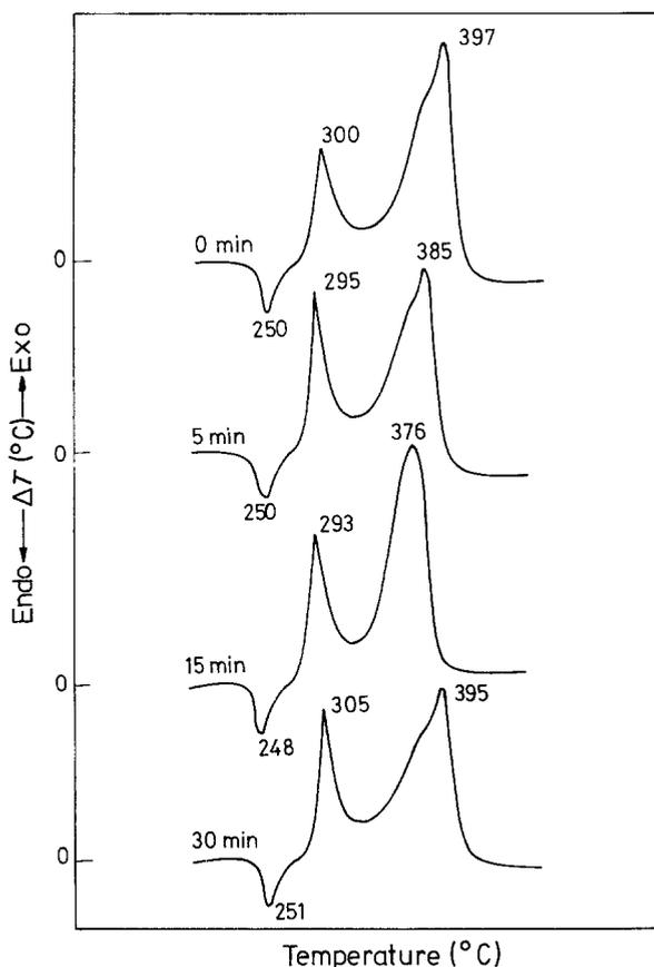
Figure 2 Differential thermal analysis curves of AP compacted at  $1500 \text{ kg cm}^{-2}$  at various dwell times. Heating rate =  $10^\circ \text{C min}^{-1}$ .
