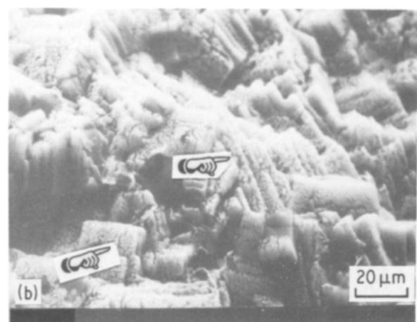
*Figure 4* SEM micrographs of quenched AP compact after partially decomposing at 310°C. (a) Microstructure of 5 min compact at 100×. Arrow indicates crack due to sudden release of product gases. Pointer indicates small decomposition nuclei at the growth stage. (b) Microstructure of Fig. 4a at a higher magnification, 1000×. Note the layered structure as indicated by a pointer. (c) Microstructure of 30 min compact at 1000×.
