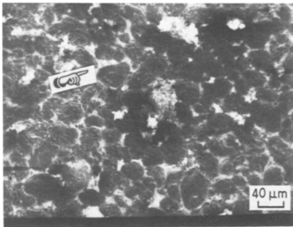
Figure 5 SEM micrograph of 50% AP-50% KP indicating melting at the grain boundaries. Compacted at  $1500 \text{ kg cm}^{-2}$  for 5 min.
