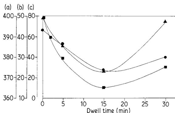
Figure 3 Representation of (a) (▲) peak temperature of the second exotherm, (b) (■)  $t_{1/2}$  from Table I and (c) (●) relative crystallite size ( $D_{211}$ ) of pellets with increase in dwell time. Note the minima observed in all the curves at 15 min dwell time.
